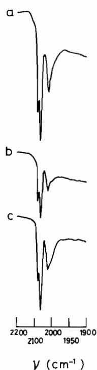
Fig. 2. Infrared spectra of \text{H}_4\text{Ru}_4(\text{CO})_{12}/\text{SiO}_2 . (a) following adsorption of \text{H}_4\text{Ru}_4(\text{CO})_{12} from heptane solution (0.24 wt.% Ru); (b) after irradiation with near-UV light in \text{N}_2 atmosphere at 25 °C for 20 h; (c) after exposure of 200 Torr CO at 70 °C for 2 hr.
